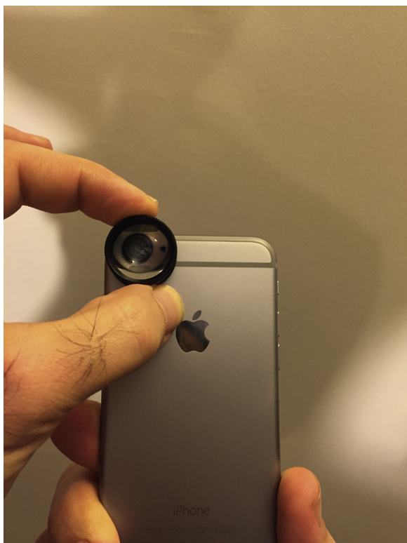
Fig. 3. The 90 Diopters lens held manually to the center of lens camera of the smartphone (iPhone 6).
